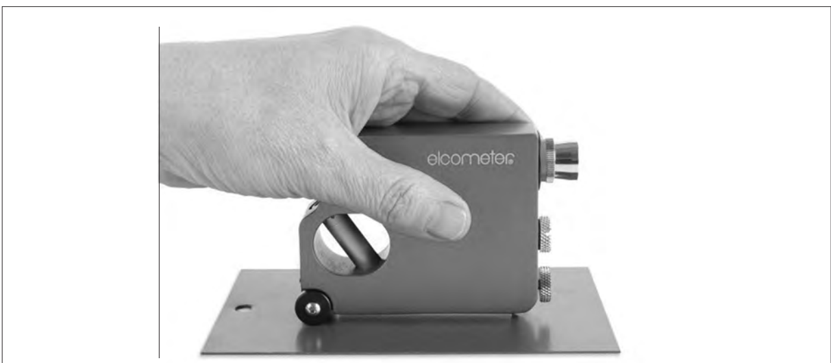
Image 7.13a The cutting tool making a V-groove incision is used for tests in accordance with ISO 2808-6B.
