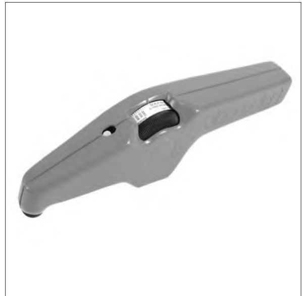
Image 7.12b The magnetic pull-off film thickness gauge is used on explosive sites, such as oil-drilling platforms, refineries and other similar facilities. The gauge is also known as the banana and is suitable for tests in accordance with ISO 2178 and ISO 2808-7A .
