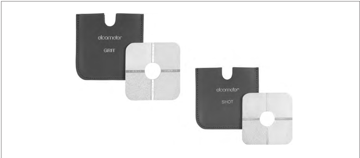
Image 4.1 ISO surface profile reference comparators for tests under ISO 8503-1 and ISO 8503-2.
