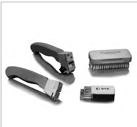
Image 8.4 Cross-cutting tool for determination of film adhesion under ISO 2409
