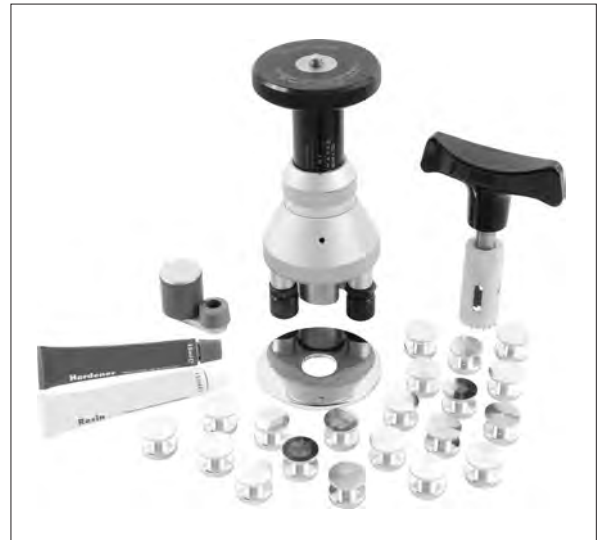
Image 8.3 Adhesion probe for measurement of film adhesion using the pull-off test under ISO 4624 and ISO 16276-1.
